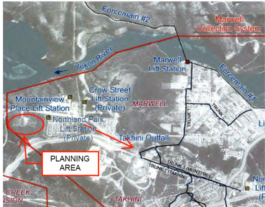
Figure 12. Range Point wastewater collection system (Source: City of Whitehorse 2003 Water and Sewer Study)
